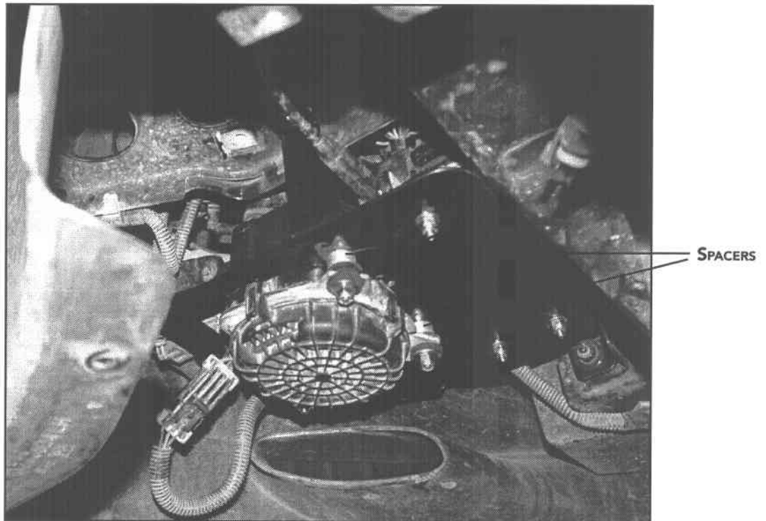
ILLUSTRATION E3 AIR PUMP AND CRUISE CONTROL RELOCATION BRACKET INSTALLED (TRANS AM WITH SPACERS INSTALLED, LOOKING UP)
