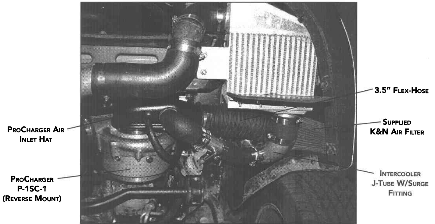
ILLUSTRATION 11 AIR INLET INSTALLED (UNDERNEATH VEHICLE, LOOKING UP)
