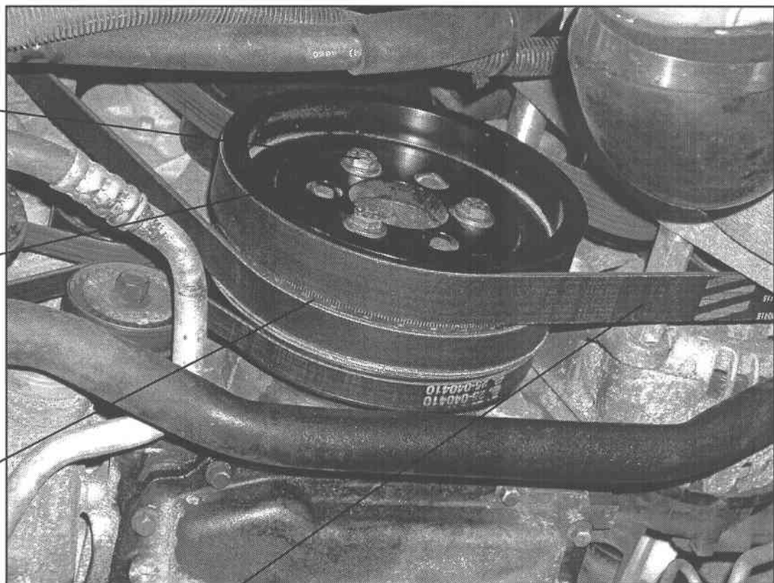
ILLUSTRATION D2 ATI PERFORMANCE PRODUCTS HARMONIC BALANCER AND 8-RIB CRANKSHAFT PULLEY INSTALLED (VIEW FROM BENEATH VEHICLE)
